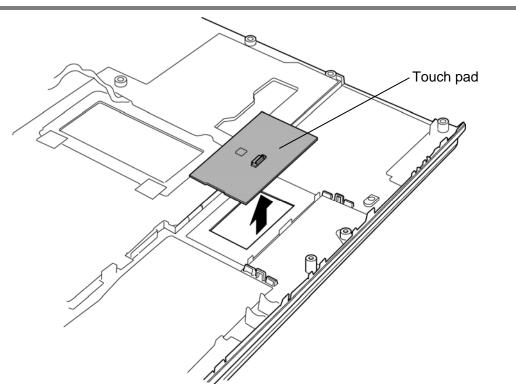
Figure 4-46 Removing the touch pad (3)
